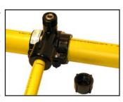
12 Line marked for stab depth should be no more than 3/4" from face of compression nut.
