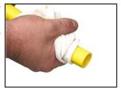
The area where the Eliminator saddle is to be installed must be cleaned to remove dirt, grease or other contamination. The elastomer seals of the Eliminator saddle should
